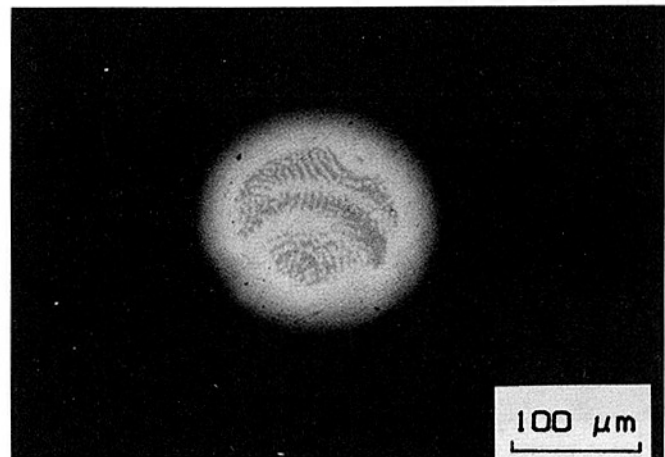
Fig. 3(e) Photograph of a polysilicon layer during melting. A circular laser beam having power P=1.6\text{ W} and 1/e irradiance radius of 60\mu\text{m} was used.
